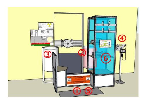
For the identified potential contamination area and contaminated area, it is necessary to set up isolation boundary. The boundaries mainly include protective equipment cabinets, barrier, dust pad and surface contamination monitoring instrument, radioactive waste collect bin and protection equipment collet bin.
