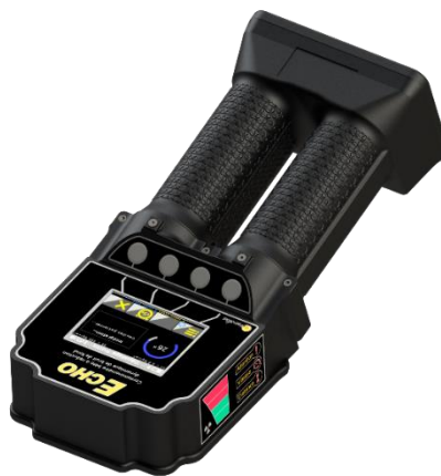
Fig. 1: photography of ECHO, an innovative device for the measurement of beta contamination in harsh environments
