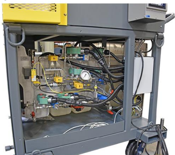
Figure 5 Coolant handling system shown on the left is in the lower portion of the module. The PLC primary control screen is on the right.
