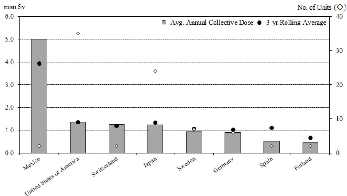
**Figure 6. 2010 PHWR average collective dose per reactor by country (man·Sv/reactor)**
